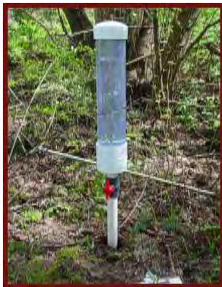
Figuur 2-21: Constant head permeameter (bron: http://www.sewagesolutions.com/permeameters.htm )
